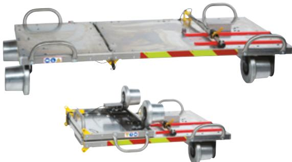
◀ Motorized trolley for aligning, stabilizing and moving the robotic welder on the track. The trolley is foldable for easy transport and fitted with a dead man's brake which blocks the wheels on both rails.
